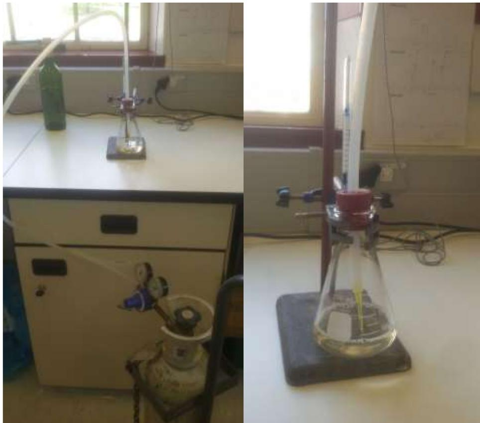
Figure 2: In-house setup for the H<sub>2</sub>S measurements
