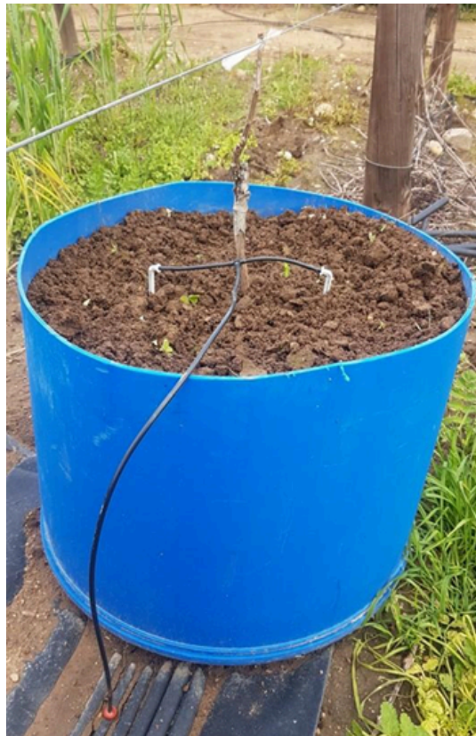
Figure 15. An image of the barbed tubing connecting the pressure-compensated dripper and the arrow dripper, as well as their placement. Note the grapevine being pruned to one cane and secured to the cordon wire.
