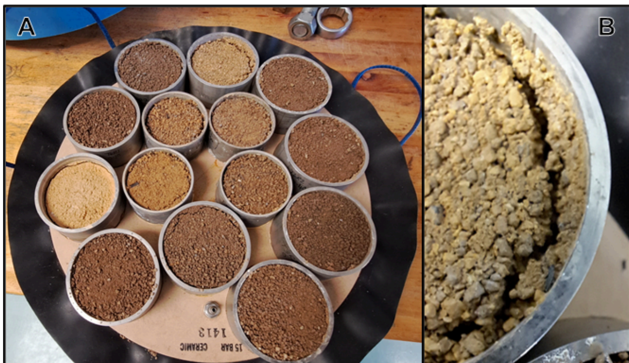
Figure 34. Examples of (A) soils with high clay contents on the pressure plate exhibiting cracks near the edges of sample rings and (B) a close-up view of a crack resulting in a preferential air flow path along the sides of the sample ring, and not through the soil sample.
