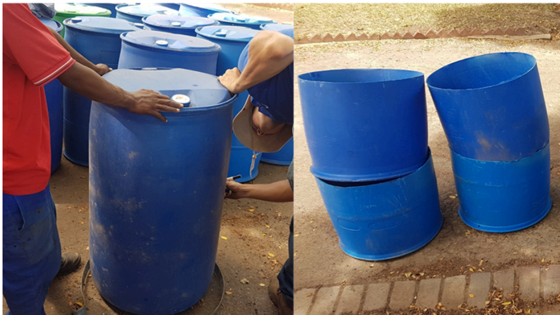
Figure 9. Polvinylchloride barrels (210 L) cut in half to create ca. 105 L pots for pot trial.
